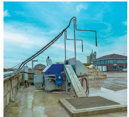
A Bibko pump discharge conveyor was installed upstream of the Bibko residual concrete recycling system, which collects the residual material from the concrete pump directly via a floor-level hopper.
