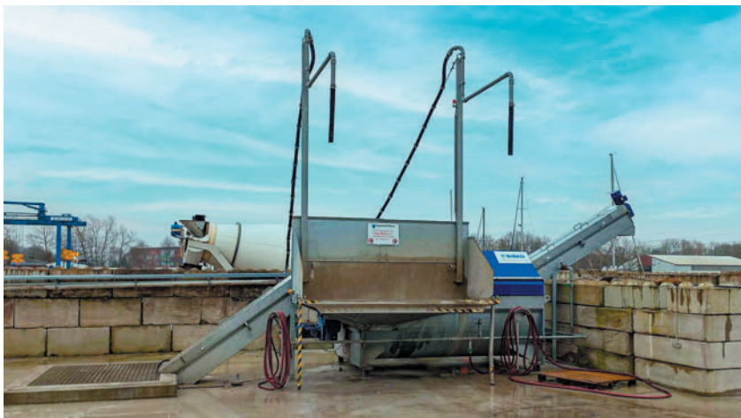
A Bibko pump discharge conveyor was installed upstream of the Bibko residual concrete recycling system, which collects the residual material from the concrete pump directly via a floor-level hopper.
