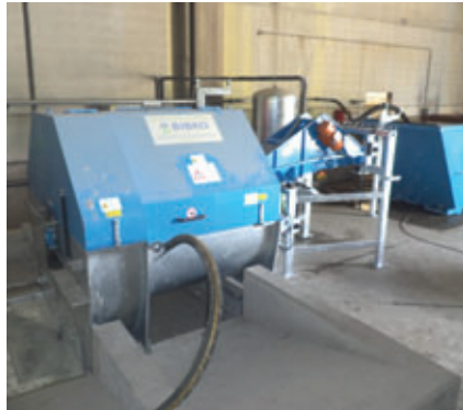
Structo NV has decided on the new ComTec 4 from Bibko for recycling residual concrete
