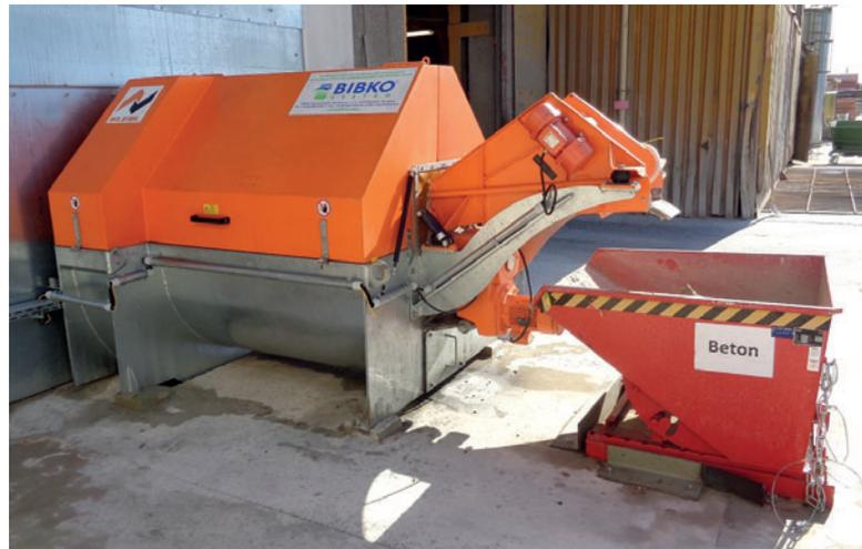
*The ComTec4 has a leaching capacity of approx. 4 m<sup>3</sup>/h and was designed mainly for precast concrete plants and smaller ready-mix concrete plants.*
