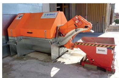
The ComTec4 has a leaching capacity of approx. 4 m³/h and was designed mainly for precast concrete plants and smaller ready-mix concrete plants.
