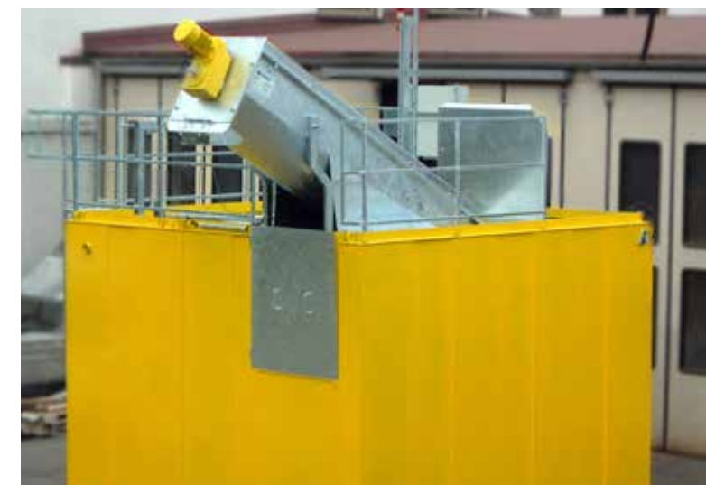
Version III: Mobile RWS in Stahlbecken integriert Mobile RWS integrated in steel tank
